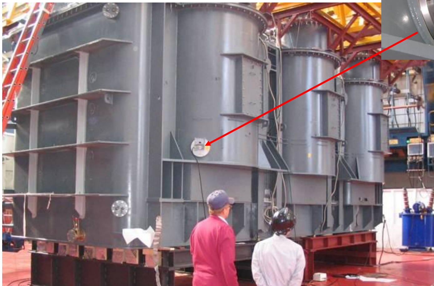
Window PD sensor fitted to a new build 400kV Series Reactor
